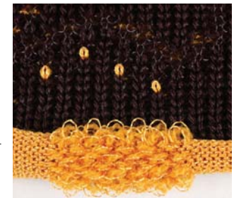
with the same machine setting you will be also enabled to knit robust plush fabrics if you think of imitating 'animal furs'
