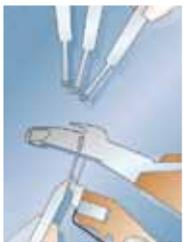
Besides, being equipped with an extra-fine compound needle system, the HKS 3-1 produces structures showing a delicate and uniform loop appearance. When fitted with an elastane device
